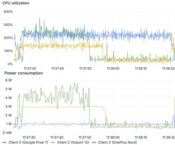
Fig. 10: CPU utilization and power consumption on heterogeneous mobile hardware. Data collected over 1 round of training on CIFAR-10 dataset.
