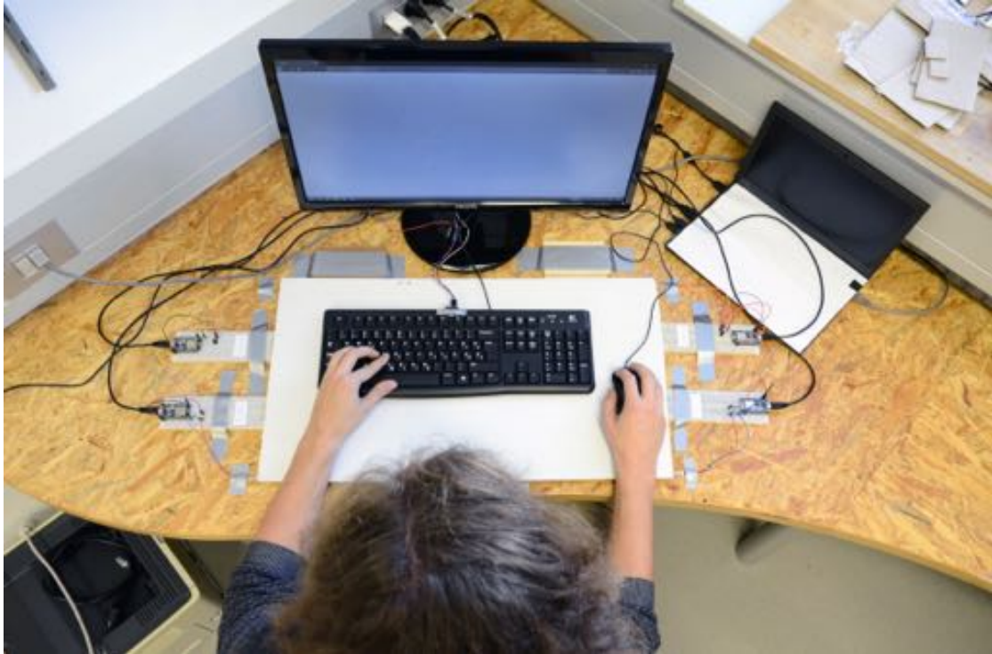
Figure 1: A participant performing the second task. Most of the environmental bed is displayed in this image – the accelerometer and gyroscope attached to the top of the keyboard, force sensors under the corners of the white pressure plate, and the PC that was used for the user study, including the PC monitor components. The only modality missing in this photo, but still present in the environment, are the infrared sensors, which are placed around the experimental environment.
