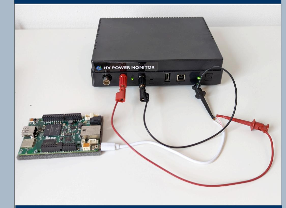
NXP™ i.MX 6SoloX applications processor with an embedded ARM Cortex-A9 core and a Cortex-M4 Core
