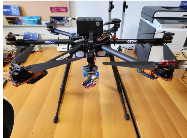
Figure 5: The UAV system designed for the AgriAdapt experiment equipped with an ArduCam camera and an NVIDIA Jetson Nano Board.
