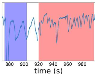
**Figure 4:** Acquired wireless signal while relaxing (blue) and solving some task (red). Unmarked (white) area is presents a time frame when user is clicking on “next slide” button and is not used in feature extraction.
