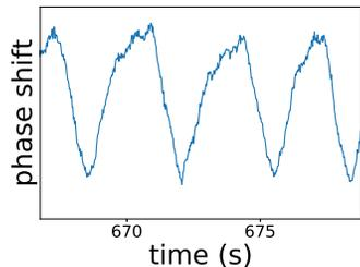
**Figure 2:** Wave phase shift of the reflected signal through time - persons inhales and exhales can be seen clearly.
