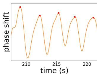
**Figure 5:** Filtered signal where each red dot/peak represents one breath. This data is later used to compute the inter-breath interval features.
