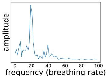
**Figure 3:** Frequency domain of the signal from Figure 2. The highest peak represent the highest probability of breathing rate.
