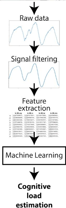
Figure 1: Wi-Mind scheme - idea for wireless cognitive load inference.
