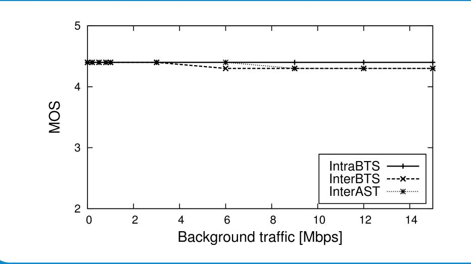
We implemented VillageCell in a lab setting and evaluated it in realistic rural-area network scenarios using traces from the Macha community network. The call quality (measured with the mean opinion score – MOS) is very good with little packet loss, fast setup time and low delay and jitter. The quality remains good even with an increasing number of simultaneous calls.
