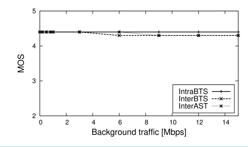
We implemented VillageCell in a lab setting and evaluated it in realistic rural-area network scenarios using traces from the Macha community network. The call quality (measured with the mean opinion score – MOS) is very good with little packet loss, fast setup time and low delay and jitter. The quality remains good even with an increasing number of simultaneous calls.
