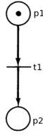
Figure 1: Example of a simple PN that describes translation. Place p_1 presents mRNA , place p_2 expressed protein and transition t_1 the reaction of translation.
