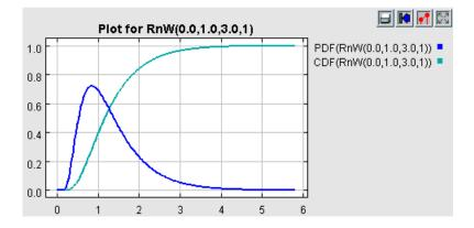
Probability density function and cumulative density function for a random walk distribution with location = 0, scale = 1, and shape = 3.
