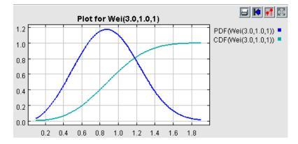
Probability density function and cumulative density function for a Weibull distribution with shape = 3 and scale = 1.
