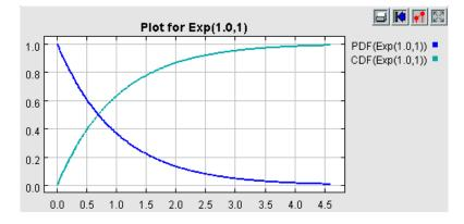
Probability density function and cumulative density function for an exponential distribution with mean = 1.
