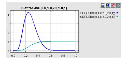
Probability density function and cumulative density function for a Johnson  $S_B$  distribution with minimum = 0, maximum = 1, shape1 = 2, and shape2 = 2.
