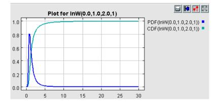
Probability density function and cumulative density function for an inverted Weibull distribution with location = 0, scale = 1, and shape = 2.
