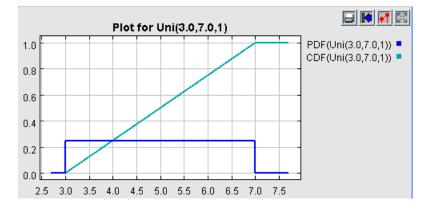
Probability density function and cumulative density function for a uniform distribution with minimum = 3 and maximum = 7.
