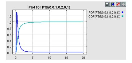
Probability density function and cumulative density function for a Pearson type V distribution with location = 0, scale = 1, and shape = 2.
