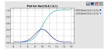
Probability density function and cumulative density function for normal distribution function with mean = 10, standard deviation = 1. There are two normal distributions in SIMPROCESS. One only returns non-negative values (zero or higher), and the other will return negative values. For both it is required that **standard deviation** > 0.0.
