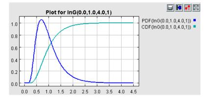
Probability density function and cumulative density function for an inverse Gaussian distribution with location = 0, scale = 1, and shape = 4.
