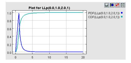
Probability density function and cumulative density function for a log-Laplace distribution with location = 0, scale = 1, and shape = 2.
