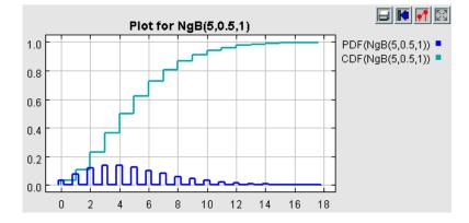
Probability density function and cumulative density function for a negative binomial distribution with s = 5 and probability = 0.5.
