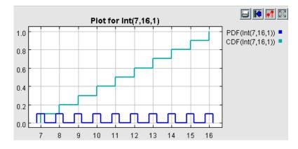
Probability density function and cumulative density function for uniform integer distribution with minimum = 7 and maximum = 16.
