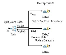
The *Original* Pad of the Split Activity is connected to the input Pad of the *Update Database* Activity, so the original customer order Entity flows through *Update Database*.
