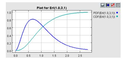
Probability density function and cumulative density function for an Erlang distribution with mean = 1 and shape = 3.
