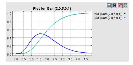
Probability density curve and cumulative density function for a gamma distribution with mean = 2 and shape = 5.
