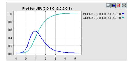
Probability density function and cumulative density function for a Johnson  $S_U$  distribution with location = 0, scale = 1, shape1 = -2, and shape2 = 2.
