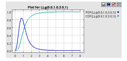
Probability density function and cumulative density function for a Log-Logistic distribution with location = 0, scale = 1, and shape = 3.
