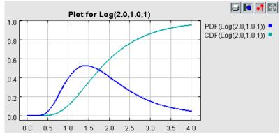
Probability density function and cumulative density function for a lognormal distribution with mean = 2 and standard deviation = 1.
