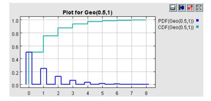
Probability density function and cumulative density function for a geometric distribution with probability = 0.5.
