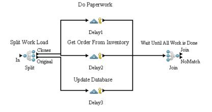
The Join Activity icon has one input Pad and two output Pads. The upper output Pad is named *Join*; Entities that are reunited with their family exit through this Pad. The lower Pad is named *NoMatch*; Entities that are not members of the Join family leave through this Pad.
