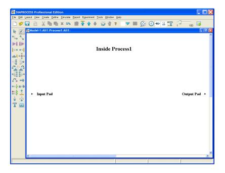
These Pads connect any Processes and Activities at this level of the sub-process to the Activities and Processes at the next higher level. Once the input and output Pad are connected by Connectors, Entities flow from level to level.
