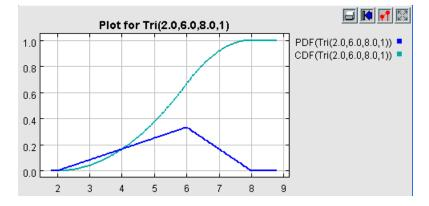
Probability density function and cumulative density function for a triangular distribution with minimum = 2, mode = 6, and maximum = 8.
