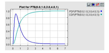
Probability density function and cumulative density function for a Pearson type VI distribution with location = 0, scale = 1, shape 1 = 3, and shape 2 = 4.
