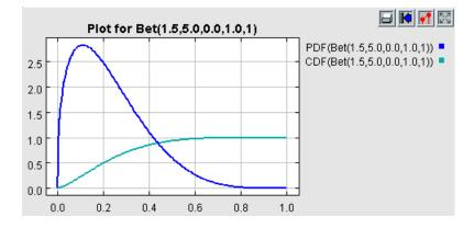
Probability density function and cumulative density function for a beta distribution with shape 1 = 1.5, shape 2 = 5.0, minimum = 0.0, and maximum = 1.0.
