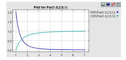
Probability density function and cumulative density function for a Pareto distribution with location = 1 and shape = 2.
