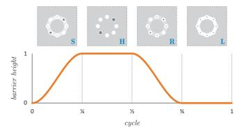
**Figure 6.** The adiabatic clock signal, which controls the cells' switching process is composed of four phases, namely: switch (S), hold (H), release (R) and relax (L). In the graph the barrier height is normalized to the interval [0, 1], where value 0 denotes lowered barriers (high probability of the electrons tunnelling between adjacent quantum dots) and value 1 denotes raised barriers (no tunnelling of electrons possible).
