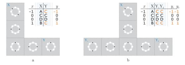
Figure 10. The corner wire and fan-out and their erroneous behaviour.
