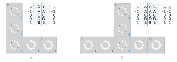
Figure 11. The pipeline architecture of corner wire and fan-out enables their correct behaviour.
