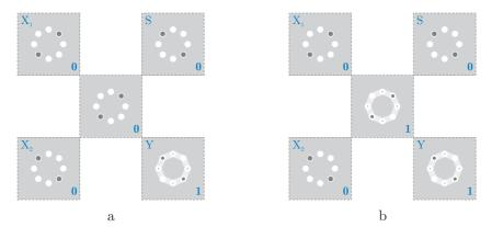
Figure 16. The two adiabatic pipeline implementations of the diagonal ternary majority voting gate.
