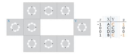
Figure 12. The erroneous behaviour of the symmetric ternary inverter.
