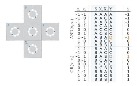
Figure 14. The QCA obtained by simple substitution of bQCA cells for tQCA cells in the binary majority voting gate and the corresponding truth table. When obeying the preconditions about the selector input S and the state D the QCA gives only two erroneous outputs.
