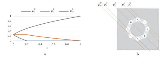
**Figure 4.** Plot of the static charge distribution (a) applied to cell X for the transition from neutral state to state A (b).
