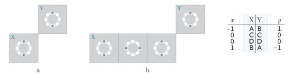
**Figure 8.** The core of ternary inverter (a) and the extension of the input section (b). The behaviour matches with the truth table of ternary negation.
