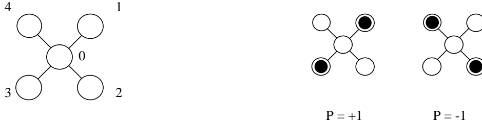
FIGURE 1. The quantum cell consisting of five quantum dots which are occupied by two electrons. The mutual Coulombic repulsion between the electrons results in bistability between the P=+1 and P=-1 states.
